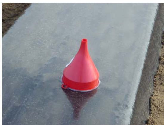
Figure 3. Plastic funnels installed to collect gas fumigants released through various mulches.
