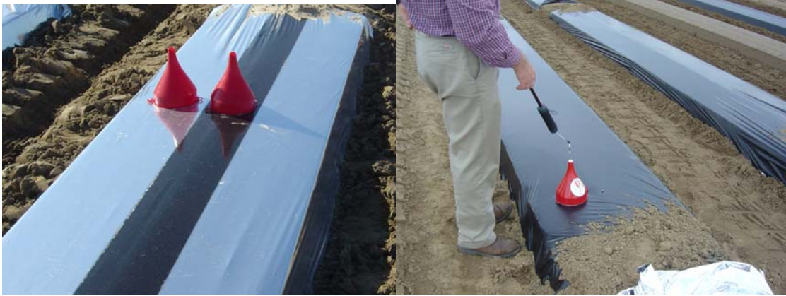
Figure 3. Plastic funnels installed to collect gas fumigants released through various mulches.
