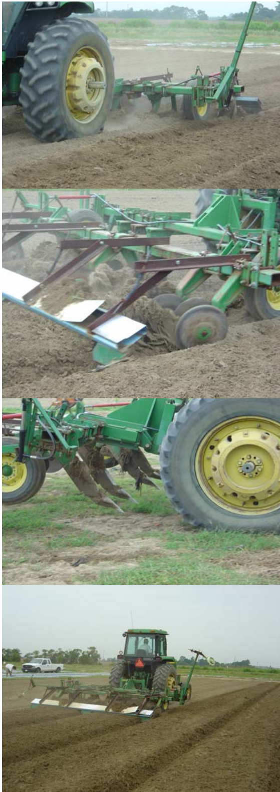
Figure 1. One pass subsoil and bed equipment.
