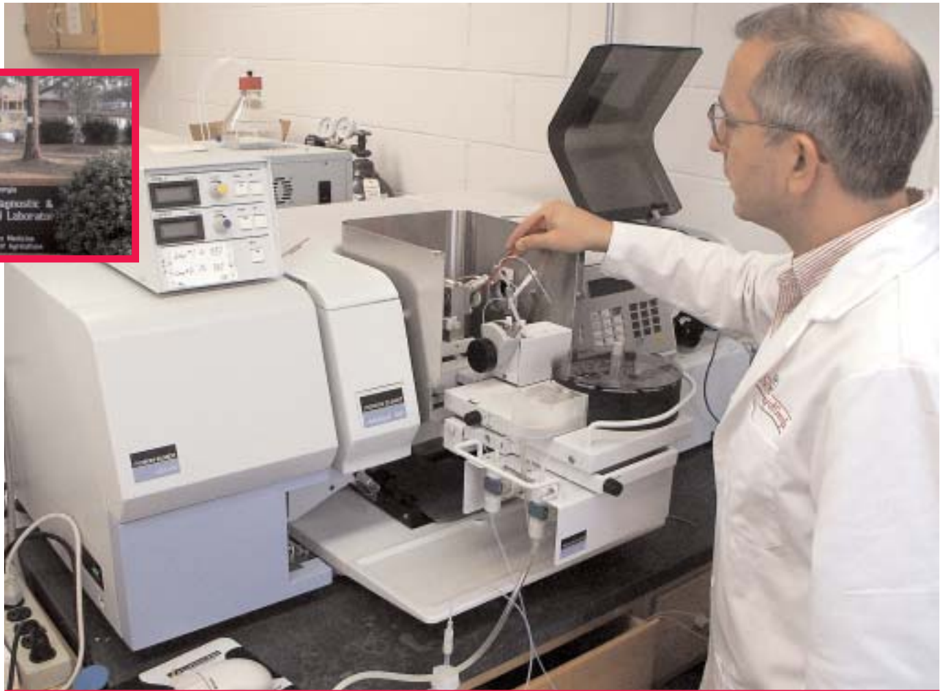
Toxicologist Larry Thompson inspects the graphite furnace of an atomic absorption spectrophotometer at the Tifton laboratory. The instrument is used for blood lead level analysis.
