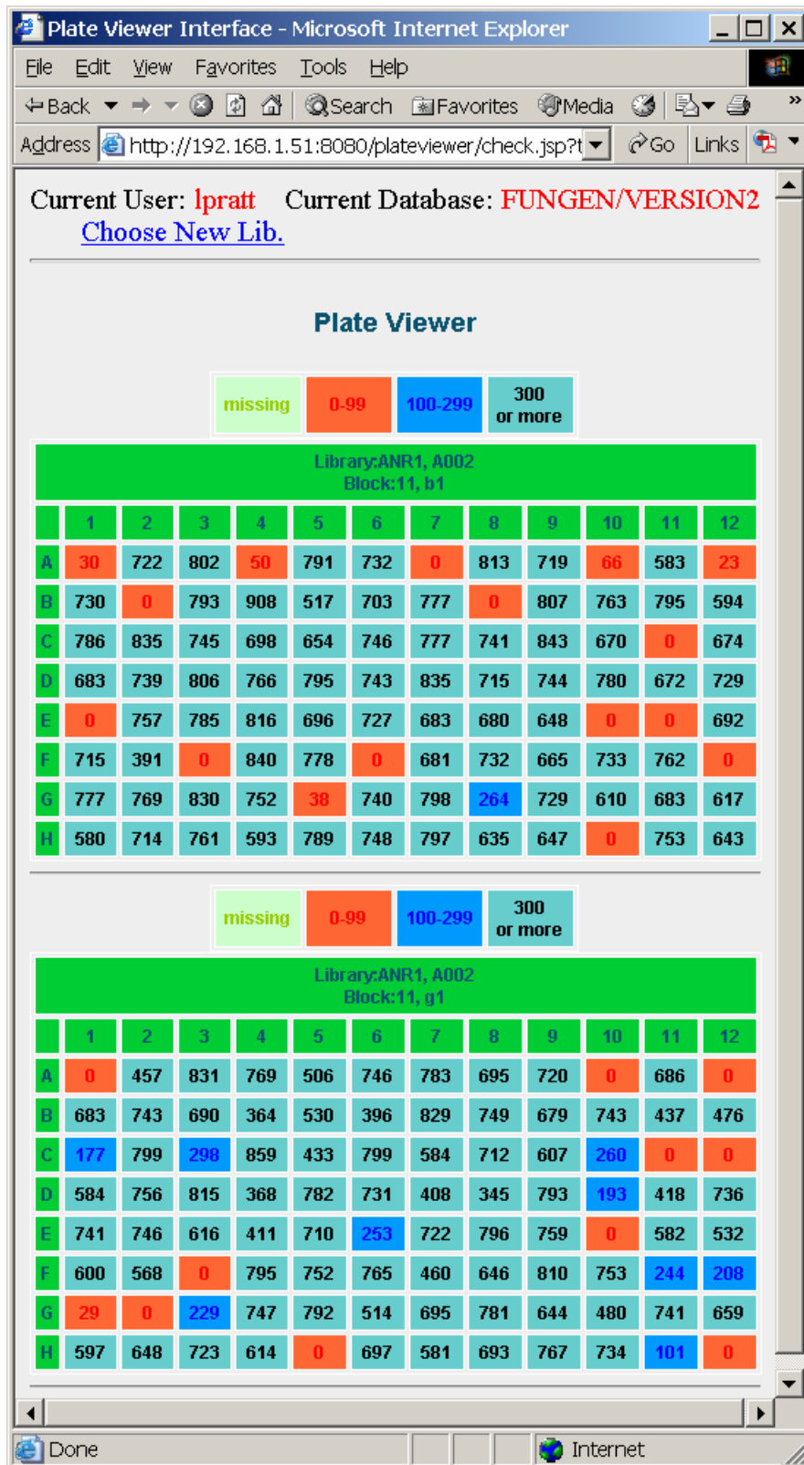
Figure 7: A screen shot of MAGIC-SPP Plate Viewer. This interface assists with troubleshooting by showing sequences from both vector directions for the same plate. For example, in this illustration wells A1, A10, A12, C11, and E10 have all failed in both forward (top) and reverse (bottom) sequencing directions indicating that these failures are most likely due to missing or poor quality template DNA. Numbers within wells represent Q16VS read lengths.
