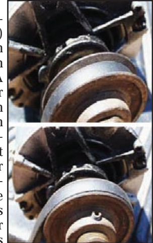
When pulleys or belts are worn, thin belts ride low in the motor pulley, as shown in top photo above. Result: blade rpm's are greatly reduced, thus robbing cfm's, air speed and wind chill cooling. Belts should be tight and ride high in the motor pulley, as in bottom photo, to achieve maximum fan rpm's and best wind-chill and evaporative cooling.
