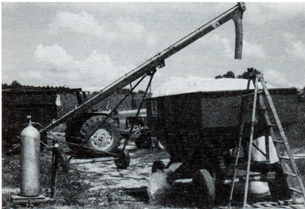
Figure 1. Corn to be treated is sealed in a plastic bag placed in a hopper bottom wagon.
